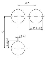
\* Recommended distance for mushroom pushbutton, emergency switch as well as position selector with protective shroud: 100 mm (3.94 in).
