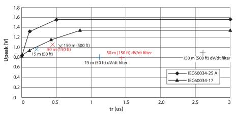
The dV/dt value decreases with the motor cable length whereas the peak voltage increases. Therefore it is recommended to use sine-wave filters in installations with motor cable lengths above 150 m (500 ft).
