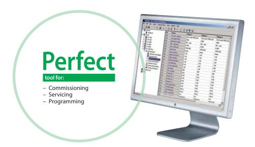
The VLT® Motion Control Tool, MCT 10, is ideal for commissioning and servicing the drive including guided programming of cascade controller, real-time clock, smart logic controller and preventive maintenance.
