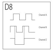
Figure 27: Reverse Quadrature A and B with ungated and inverted Index centered on B low between 360° and 180°
