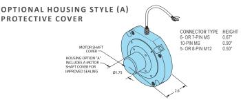
All dimensions are in inches with a tolerance of +0.005" or +0.01" unless otherwise specified.
