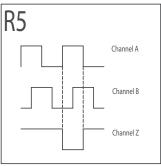
Figure 5: Quadrature A and B with inverted 180° Index gated to A
