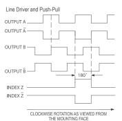
NOTE: ALL DEGREE REFERENCES ARE ELECTRICAL DEGREES. WAVEFORM SHOWN WITH OPTIONAL COMPLEMENTARY SIGNALS Ā, Ē, Ž FOR HV AND H5 OUTPUTS ONLY
