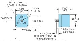
All dimensions are in inches with a tolerance of  $\pm 0.005$ " or  $\pm 0.01$ ". unless otherwise specified metric dimensions are given in brackets [mm].
