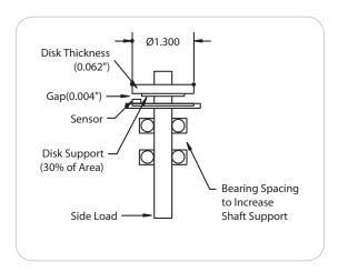
doubled from 0.002" to 0.004", and the disk diameter was reduced from 2.0" to 1.3".
