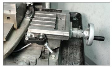
The TR2 is ideal for gauging and backstop applications typically found on a variety of metal working equipment.
