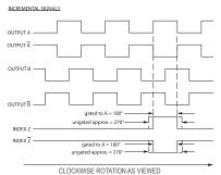
FROM THE MOUNTING FACE NOTE: ALL DEGREE REFERENCES ARE ELECTRICAL DEGREES WAVEFORM SHOWN WITH OPTIONAL COMPLEMENTARY SIGNALS  $\overline{A}$ ,  $\overline{B}$ ,  $\overline{Z}$  FOR HV AND H5 OUTPUTS ONLY.
