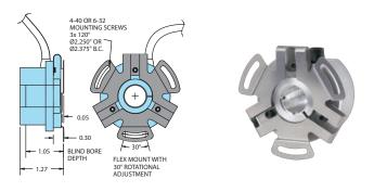
All dimensions are in inches with a tolerance of  $\pm 0.005$ " or  $\pm 0.01$ " unless otherwise specified.
