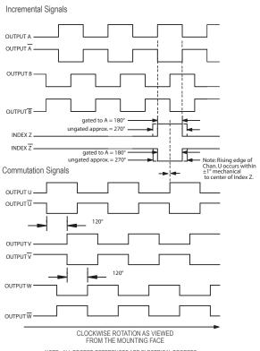
NOTE: ALL DEGREE REFERENCES ARE ELECTRICAL DEGREES. WAVEFORM SHOWN WITH OPTIONAL COMPLEMENTARY SIGNALS Ā, Ē, Z̄ FOR HV AND OD OUTPUTS ONLY.
