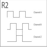
Figure 12: Quadrature A and B with 180° Index gated to B low
