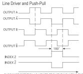
CLOCKWISE ROTATION AS VIEWED FROM THE MOUNTING FACE NOTE: ALL DEGREE REFERENCES ARE ELECTRICAL DEGREES WAVEFORM SHOWN WITH OPTIONAL COMPLEMENTARY SIGNALS Ā, Ē, Z FOR HV OUTPUT ONLY.
