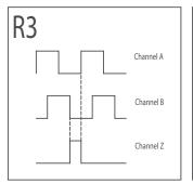
Figure 13: Quadrature A and B with 90° Index gated to A low and B low
