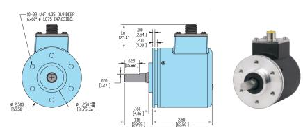
All dimensions are in inches with a tolerance of  $\pm 0.005$ " or  $\pm 0.01$ " unless otherwise specified. Metric dimensions are given in brackets [mm].
