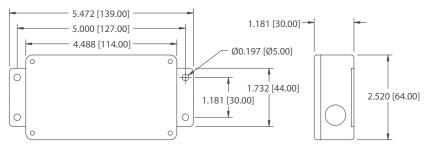
All dimensions are in inches with a tolerance of  $\pm 0.005$ " or  $\pm 0.01$ " unless otherwise specified. Metric dimensions are given in brackets [mm].
