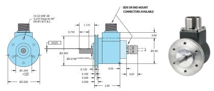
All dimensions are in inches with a tolerance of  $\pm 0.005$ " or  $\pm 0.01$ " unless otherwise specified.
