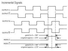
CLOCKWISE ROTATION AS VIEWED FROM THE SHAFT SIDE (FOR UNITS WITH DUAL WHEELS, ORIENT THE ENCODER SO THAT THE LABEL IS READABLE).
