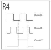
Figure 8: Quadrature A and B with ungated Index centered on A between 360° and 180°
