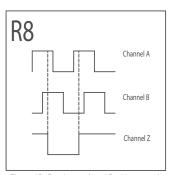
Figure 18: Quadrature A and B with ungated inverted Index centered on A low between 360°
