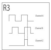
Figure 4: Quadrature A and B with 90° Index gated to A and B
