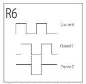
Figure 16: Quadrature A and B with inverted 180° Index gated to B low
