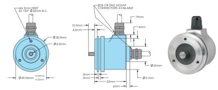
All dimensions are in millimeters with a tolerance of ±0.17 mm unless otherwise specified.
