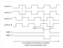
NOTE: ALL DEGREE REFERENCES ARE ELECTRICAL DEGREES WAVEFORM SHOWN WITH OPTIONAL COMPLEMENTARY SIGNALS Ā, B, Z FOR HV OUTPUT ONLY.
