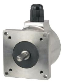
Industry Standard Size 20 (2" Diameter) Stainless Steel Package Flange and Servo Mounting Up to 30,000 CPR 80 lb Maximum Axial and Radial Shaft Loading **IP67 Sealing Available**
