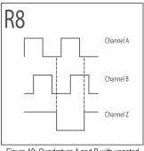
Figure 10: Quadrature A and B with ungated inverted Index centered on A between 360° and 180°
