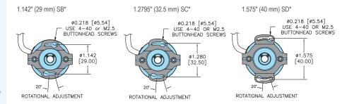
\*Order Appropriate No Charge Mounting and Installation Kit for SB, SC, or SD Option. Each kit contains 10 screws for mounting 5 encoders.
