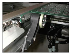
For linear applications, the Tru-Trac™ can be mounted above or below the moving object, and the tension on the wheel can be adjusted for a wide range of applications, such as packaging, conveyors, mail sorting, cut-to-length, labeling, gantries, etc.
