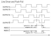
CLOCKWISE ROTATION AS VIEWED FROM THE MOUNTING FACE NOTE: ALL DEGREE REFERENCES ARE ELECTRICAL DEGREES. VAVEFORM SHOWN WITH OPTIONAL COMPLEMENTARY SIGNALS  $\bar{A}$ ,  $\bar{B}$ ,  $\bar{Z}$  FOR HV OUTPUT ONLY.
