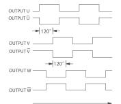
CW ROTATION OF SHAFT AS VIEWED LOOKING AT THE ENCODER FACE. NOTE: ALL DEGREE REFERENCES ARE ELECTRICAL DEGREES.
