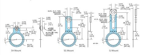
All dimensions are in inches with a tolerance of  $\pm 0.005$ " or  $\pm 0.01$ " unless otherwise specified.
