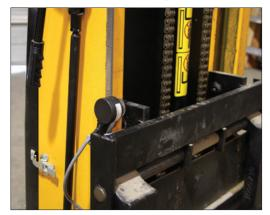
The Model TR2 is applied to provide vertical speed and position feedback for a fork lift tower.
