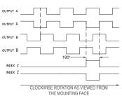
NOTE: ALL DEGREE REFERENCES ARE ELECTRICAL DEGREES. WAVEFORM SHOWN WITH OPTIONAL COMPLEMENTARY SIGNALS Ā, Ē, Z̄ FOR HV AND H5 OUTPUTS ONLY.
