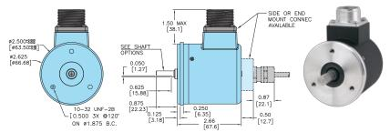
All dimensions are in inches with a tolerance of  $\pm 0.005$ " or  $\pm 0.01$ " unless otherwise specified.
