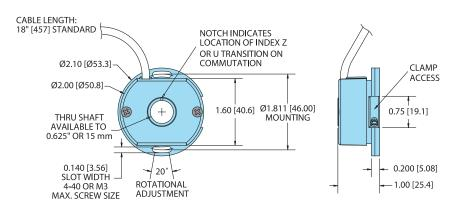
All dimensions are in inches with a tolerance of +0.005" or +0.01" unless otherwise specified Metric dimensions are given in brackets [mm].
