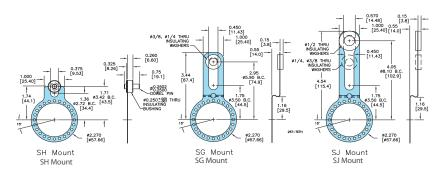
All dimensions are in inches with a tolerance of +0.005" or +0.01" unless otherwise specified. Metric dimensions are given in brackets [mm].
