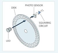
Resolution is a term used to describe the Cycles Per Revolution (CPR) for incremental encoders. Each incremental encoder has a defined number of cycles that are generated for each 360 degree revolution of the shaft. These cycles are monitored by a counter or motion controller and converted to counts for position or velocity control. The diagram shows how the whole encoder comes together.
