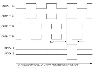
NOTE: ALL DEGREE REFERENCES ARE ELECTRICAL DEGREES. COMPLEMENTARY SIGNALS  $\overline{A}, \overline{B}, \overline{Z}$  APPLY TO LINE DRIVER (HV & H5) OUTPUTS ONLY.
