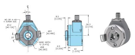
Primary dimensions are in mm, secondary dimensions SI units [inches] in brackets for reference only.
