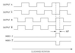
NOTE: ALL DEGREE REFERENCES ARE ELECTRICAL DEGREES. WAVEFORM SHOWN WITH OPTIONAL COMPLEMENTARY SIGNALS  $\overline{A}, \overline{B}, \overline{Z}$  FOR HV OUTPUT ONLY.
