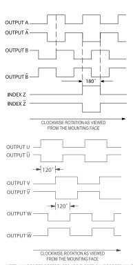
NOTE: ALL DEGREE REFERENCES ARE ELECTRICAL DEGREES WAVEFORM SHOWN WITH OPTIONAL COMPLEMENTARY SIGNALS Ā, Ē, Ē FOR HV AND OD OUTPUTS ONLY.
