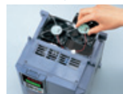
Disconnect the power connector and change the cooling fan cartridge.
