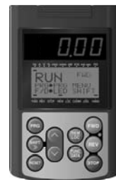
Figure 4.2 Display of the LED Monitor after Power-on
