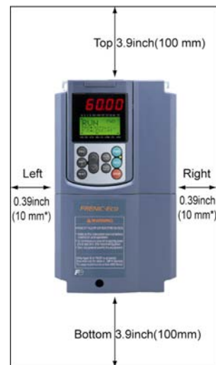
Figure 2.1 Mounting Direction and Required Clearances
