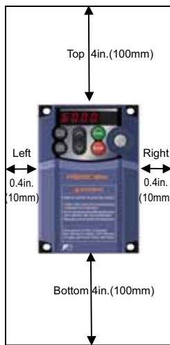
Figure 2.1 Mounting Direction and Required Clearances
