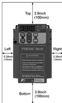
Figure 2.1 Mounting Direction and Required Clearances
