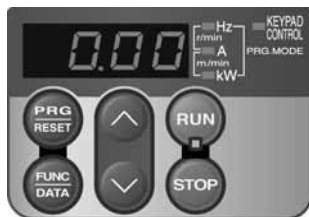
Figure 4.2 Display of the LED Monitor after Power-on
