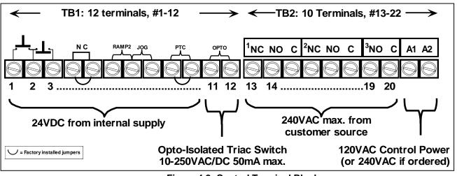
Figure 4.2: Control Terminal Blocks
