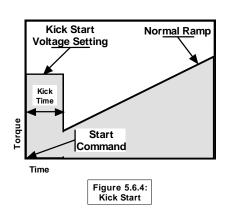
Kick Start applies a pulse of voltage to the motor producing a momentary "kick" of high torque to break the motor load free from high friction or frozen components. This pulse is limited to 2 seconds.
