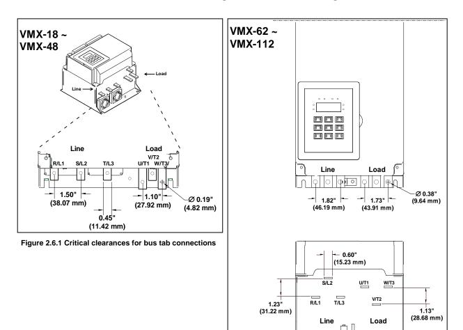
Figure 2.6.2 Critical clearances for bus tab connections
