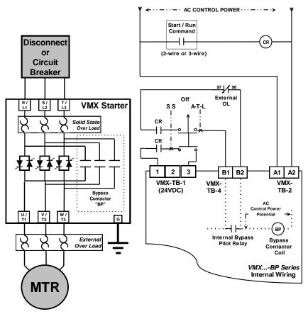
Figure APP5.2: VMX Wiring for Across-the-Line Bypass Operation with External Overload Relay (Only the terminals necessary for this operation are shown)
