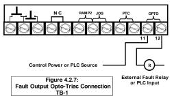
An optically isolated Triac output is dedicated as a fault indicator on TB1, terminals 11 and 12, labeled "**Opto**". The output Triac switch is rated for 10 - 250 VAC/DC, **50 mA (maximum)**. If the three programmable Output Auxiliary Relays are being used for other functions, this output can easily be hooked up to a PLC or small external relay to provide a Fault signal. This Fault Output operation is permanently fixed at "Any Trip", duplicating the Relay setting 16 as shown in Table 5.6.10.
