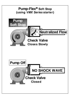
Pump-Flex<sup>®</sup> Deceleration (Soft Stop) is a unique feature of Motortronics Solid State Soft Starters. It provides a slow decrease in the output voltage, accomplishing a gentle decrease in motor torque during the stopping mode. This is the **OPPOSITE OF BRAKING** in that it will take **longer** to come to a stop than if the starter were just tuned off.
