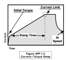
**3. Closed Loop Current (Torque) Ramping** provides smooth linear acceleration of output torque. Ramp Time becomes the time from Initial Torque and Current Limit settings. Output torque is constantly updated using an internal PID feedback loop to provide a linear ramp, therefore the available torque is maximized at any given speed. The best use of this feature is for applications where rapid changes in torque may result in load damage or equipment changes. Examples would be:
