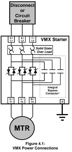
\*Larger units (210A and above) can be ordered with fan cooling instead of Bypass Contactors, but are intended for use in NEMA 1 ventilated enclosures only. Do not use the VMX starter in a sealed enclosure without a bypass contactor.
