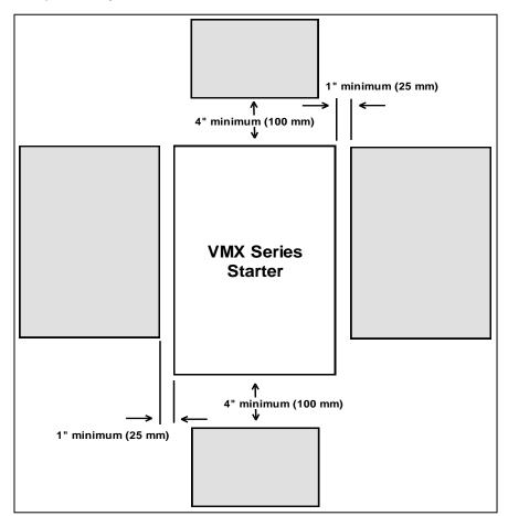
Figure 2.5: VMX minimum mounting clearances
