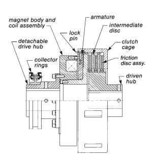
Torque 600 to 9000 lb-ft Basic Unit (as shown) Form 1
