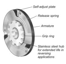
Gap system maintains a consistent deenergized armature-to-friction-face air gap. This spacing is automatically adjusted with each armature engagement throughout the useful life of the product.
