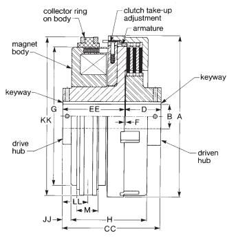
Style E Clutch with collector ring on magnet body. Driven hub Form 1.
