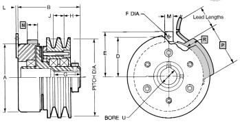
Lead Lengths: All Tor-ac units have 32" leads. Standard DC unit has 24" leads.
