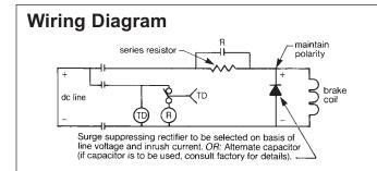
(R) is a normally open, single pole, DC contactor. (TD) is a normally closed time delay relay.
