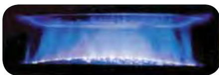
Axial Magnetic Field Interrupter - Arc Dispersion
