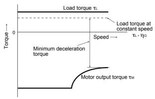
Fig. 4.5 Example study of minimum deceleration torque (1)
