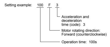
Set the operation time to 0.00 for stages not used, which are skipped in operation.
