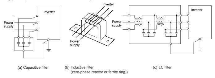
Fig. 10 Various filters and their connection methods
