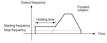
The operation does not start when the starting frequency is less than the stop frequency or when the setting frequency is less than the stop frequency.
