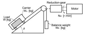
Fig. 4.9 Moving a load along a slope
