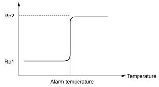
The figure in "H26 PTC thermistor (Mode select)," shows that resistor  $250\Omega$  and the thermistor (resistance value Rp) are connected in parallel. Hence, voltage  $V_{\text{C1}}$  (operation level) at terminal C1 can be calculated by using the following formula.
