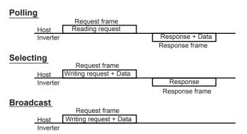
**Description) Broadcast** (selecting one lump of all terminals) A frame set with station address of 99 is treated by all inverters as broad cast. By using broadcast, operation commands and frequency command can be give all the inverters in a lump. (The writing of S01 - S06 ['W', 'E' commands] in the standard frame and 'a' - 'f' and 'm' commands in the option frame are only valid.)
