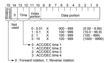
Example) If "C22:Stage1" = 10.0s R2 (10s, reverse rotation, acceleration time 2/deceleration time 2),
