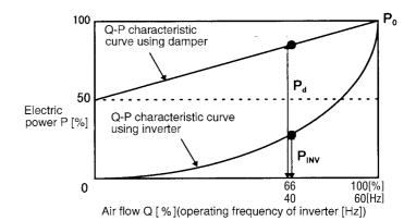
Fig.1 Q-P characteristic curve
