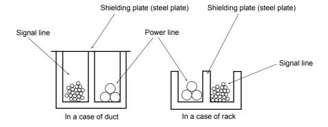
Fig. 7 Method of separating wiring
