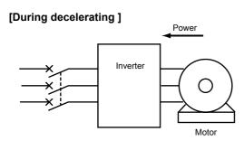
If the time for decelerating an inverter is set shorter than the natural stopping time for a load machine, the motor works as a generator when it decelerates, causing the kinetic energy of the load to be converted to electric energy that is returned to the inverter from the motor. If this power (regenerative power) is consumed by the inverter, the motor generates a braking force called "braking torque."
