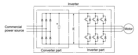
Fig. 1 Main circuit configuration of inverter
