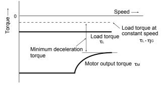
Fig. 4.6 Example study of minimum deceleration torque (2)
