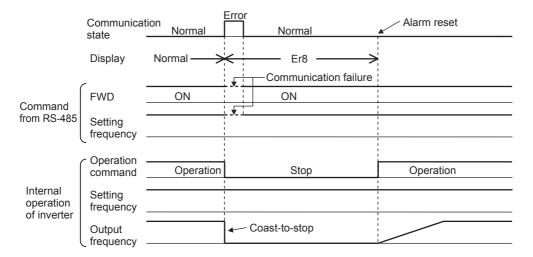
In a case of H32=1, H33=5.0s (Mode of immediate forced stop after 5s at occurring communication error)
