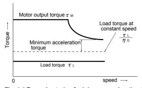
Fig. 4.4 Example study of minimum acceleration torque
