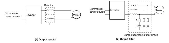
Fig. 4 Method to suppress surge voltage
