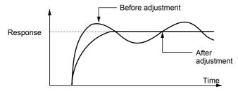
To suppress vibration with a frequency roughly equivalent to the value "H24 D-gain," decrease the value of H24. If there is residual vibration with 0.0, decrease the value of "H22 P-gain."
