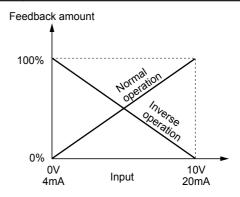
Only positive values can be input for this feedback amount of PID control. Negative values (e.g., 0 to -10V, -10 to 0V) cannot be input, thereby the function cannot be used for a reverse operation by an analog signal.
