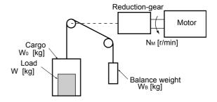
Fig. 4.8 Moving a load vertically
