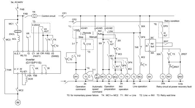
Inverter retry and restart sequence after momentary power failure and power recovery (Example 2) (Inverter → Commercial power → Inverter, Automatic changeover sequence: Using inverter built-in sequence)
