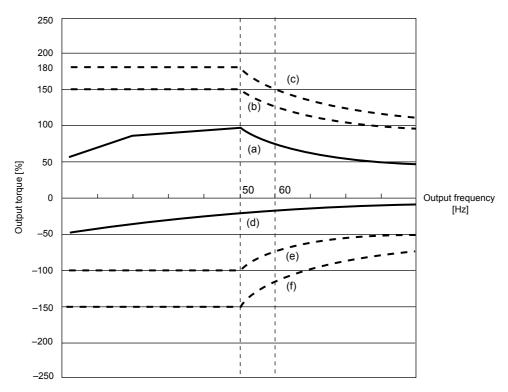
Fig. 4.1 Output torque characteristics (50Hz base)
