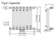
The capacitor for the filter OFL-30-4A or larger has to be installed separately. (The capacitor mass is not included in the filter mass on the table below.)
