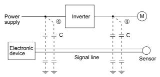
Fig. 5 Electrostatic noise
