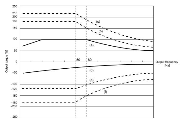
Fig. 4.2 Output torque characteristics (60Hz base)
