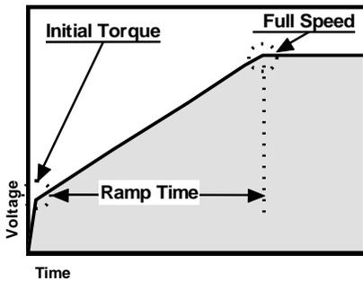
Figure APP 1.1: Voltage Ramp w/o Current Limit
