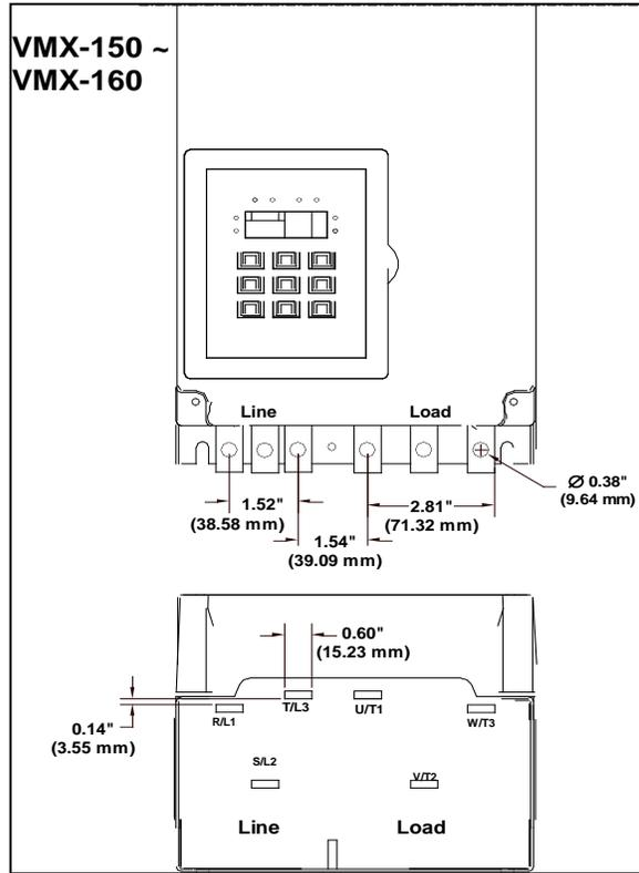
Figure 2.6.3 Critical clearances for bus tab connections
