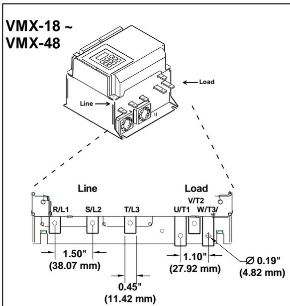
Figure 2.6.1 Critical clearances for bus tab connections
