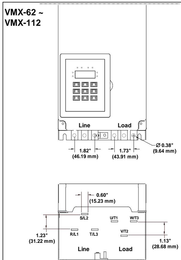
Figure 2.6.2 Critical clearances for bus tab connections
