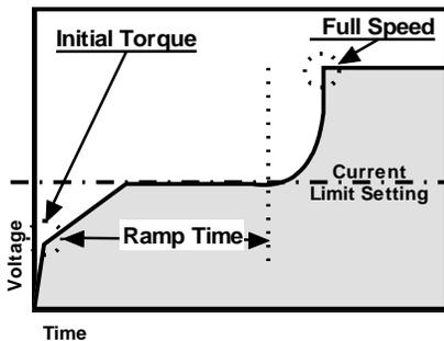
Figure APP 1.2: Voltage Ramp with Current Limit
