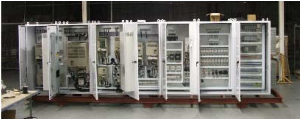
The panel includes 9 AC vector drives, from 2 to 150 hp, with common DC bus for load sharing applications. The drives control the entire machine from the drawbox, where a wire rod is drawn down to fine wire, to the dual spooler where the fine wire is wound on reels for shipment to the customer. The panel also includes a complete PLC system and motor starters for all of the auxiliary controls required for the machine.
