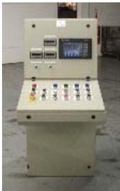
The operators control console, with a 256 x 128 pixel interface screen, gives the operator a single station where he can monitor and control the entire machine.
