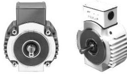
See Page 15 for ordering. The 20 Module mounts directly to a C-face motor and can then mount to a C-face reducer. It can also be direct coupled or used to connect driven equipment by belt or chain. It is a power-on brake. External dimensions are identical with most competitive brands making field replacements an exact "drop-in." No component assembly required. Washdown models now available in select sizes.
