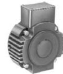
See Page 16 for ordering. The 20MB Module is a power-on brake. It is designed to be mounted on the accessory end of a double-shafted, C-face motor. External dimensions are identical with most competitive brands making field replacement an exact "drop-in." No component assembly required.
