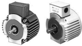
See Page 13 for ordering. The 1020 Module mounts directly to a C-face motor and can then mount to a C-face gear reducer. It can also be direct coupled or used to connect driven equipment by belt or chain. Both the clutch and brake elements are power-on for activation. External dimensions are identical with most competitive brands making field replacement an exact "drop-in." No component assembly required. Washdown models now available in select sizes.
