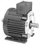
See Page 14 for ordering. The 3040B Module is a foot or base-mounted clutch-only unit. It can be direct coupled in a drive system or connected through belt and/or chain equipment. The 3040 and 3040B models can be user built-up from 1040 Modules by adding on the input adapter kit (3040) and the base kit with the input adapter kit (3040B).
